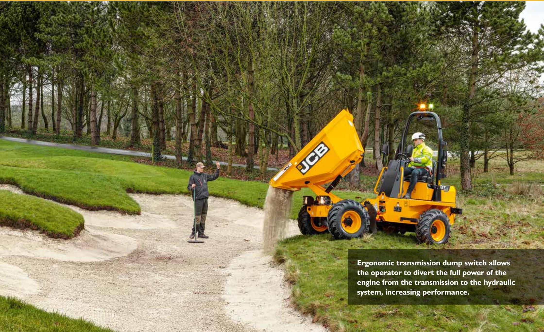
**Ergonomic transmission dump switch allows the operator to divert the full power of the engine from the transmission to the hydraulic system, increasing performance.**
